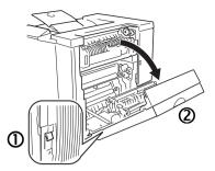
*If you have lower feeder unit attached, you first need to open the lower right-side door.*
